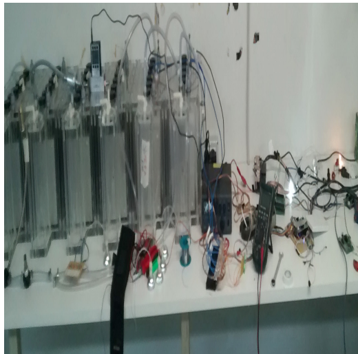
Figure 1: Construction and programming HHO Cells
