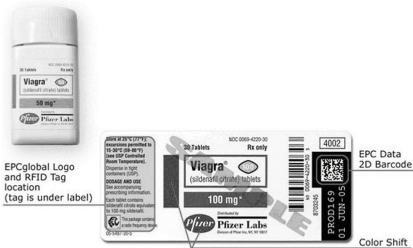
Figure 1. Anti-counterfeit measures for protection of one of Pfizer's most known brands, Viagra ®16
