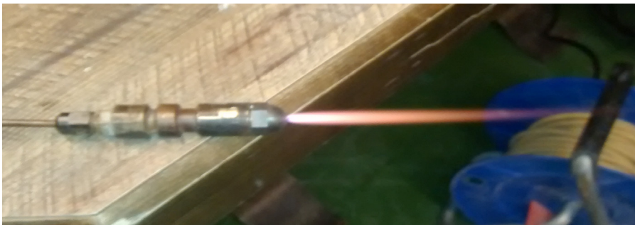
Figure 4: The flame of the burner uses only 750W of electricity.
